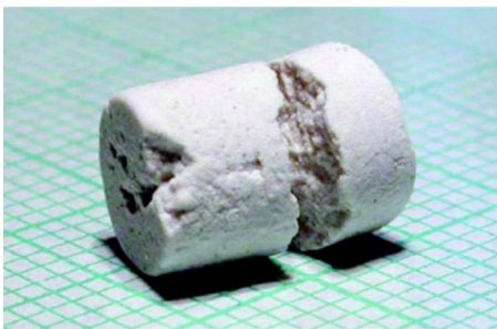
FIG. 2. (Color online) Typical fracture pattern for a U30 model stone treated fixed at the focus of an HM-3 clone lithotripter. The proximal face (left) has cavitation pitting. The stone is fractured in two pieces about 1/3 of the length from the distal end.
