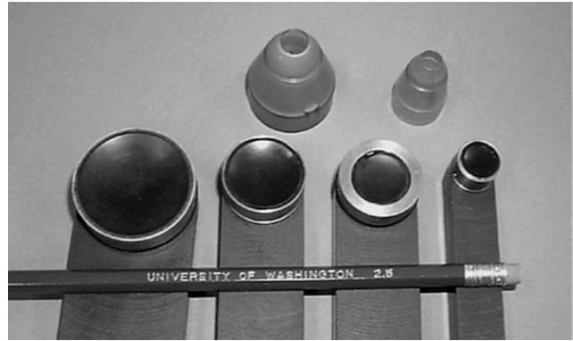
**Fig. 2.** Single element piezoceramic transducers (3–10 MHz) designed for acoustic hemostasis. The circular matching layer and element connect to a 10-cm handle. A detachable water-filled cone provides the acoustic coupling. [Figure courtesy of P.J. Kaczkowski, CIMU, University of Washington.]
