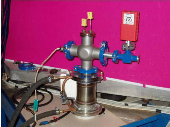
Fig. 4. The high-temperature furnace on HRFD, FNLP, Dubna, Russia. The height of the furnace section is about 10 cm.
