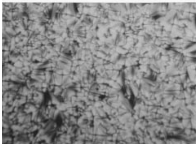
Figure 3. Polarized optical micrographs of the SA mesophase textures observed after annealing for 1 h upon cooling copolymers from the isotropic melt: (a) 140.0 °C, copolymer AX with 70 mol % of the chiral units; (b) 120.0 °C, copolymer BX with 60 mol % of the chiral units (200 \times ).
