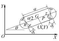
Under these conditions velocities of the points F and R will be directed horizontally and perpendicularly to the axles of the wheels and there is a point P on the line FR which has zero lateral velocity. Its forward velocity we denote by u. It may be shown, that (see e.g. [5, 6, 7, 8, 13])
