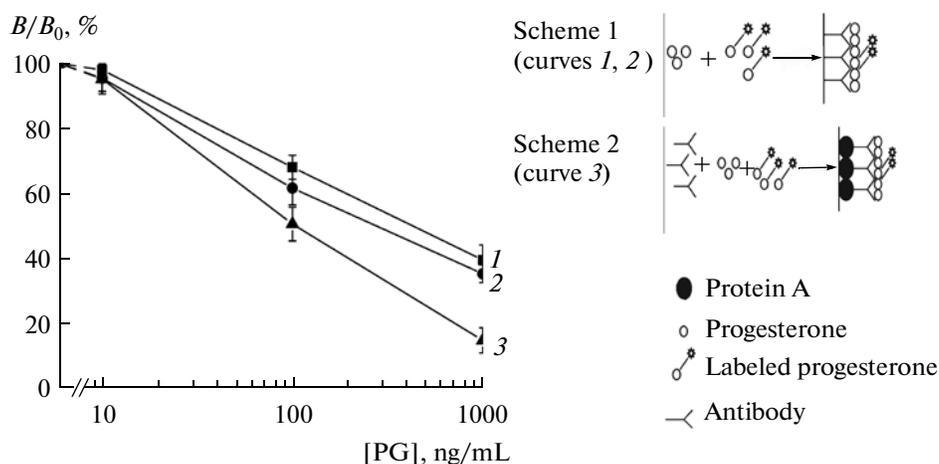
**Fig. 2.** Calibration curves for PG detection using LFIA employed colloidal gold as a label. Gold particles with a size 16 nm (1) and 35 nm (2, 3) were employed in LFIA according to schemes 1 (1, 2) and 2 (3).
