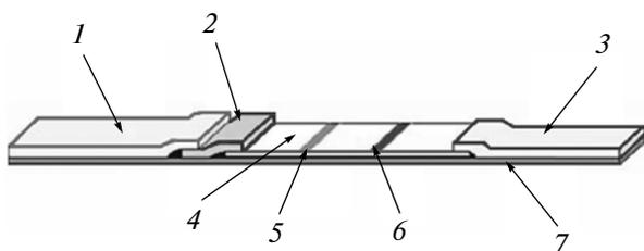
**Fig. 1.** Construction of a test strip for LFIA. 1—sample pad; 2—conjugate pad; 3—absorbent pad; 4—analytical membrane; 5—test band; 6—control band; 7—plastic base.
