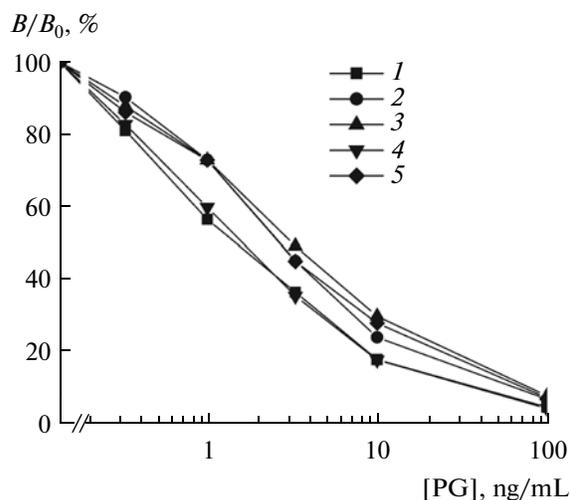
**Fig. 4.** Calibration curves for PG detection by ELISA using the following working buffers: 1—PBS; 2—PBS containing 0.05% Tween-20, 10% sucrose; 3—PBS containing 0.05% Tween-20, 0.1% BSA; 4—PBS containing 10% sucrose, 0.1% BSA; 5—PBS containing 0.05% Tween-20, 10% sucrose, 0.1% BSA.
