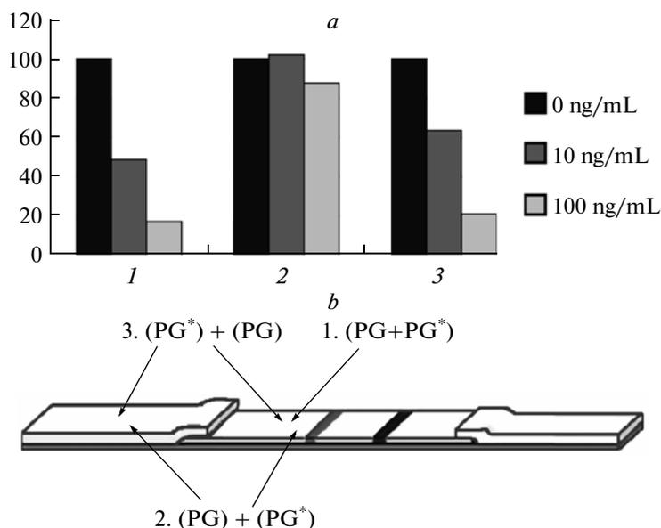
**Fig. 5.** Curve of color staining of analytical zone of a membrane on PG concentration for different sequences of reagent loading using LFIA employed enzyme as a label.
