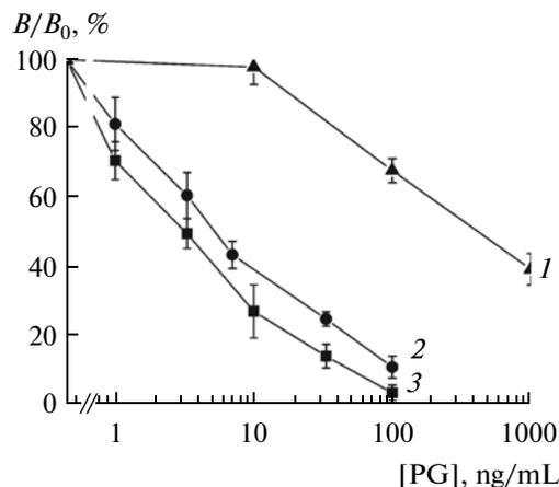
**Fig. 8.** Calibration dependences for PG detection using various methods as follows: 1—LFIA employed colloidal gold as a label; 2—LFIA using horseradish peroxidase as a label; 3—ELISA.
