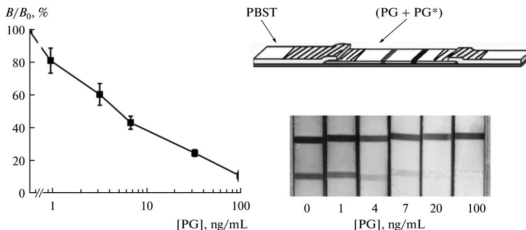
**Fig. 7.** Scheme of analysis, calibration curve and result of signal visualization for detecting PG using LFIA employed enzymatic labeling. Area of lamination is patterned.
