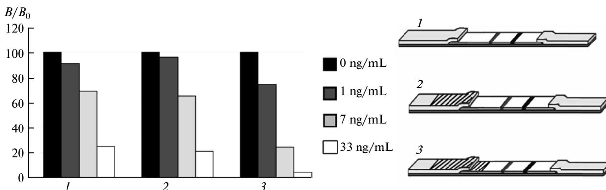
**Fig. 6.** Curve of color staining of analytical zone of membrane on PG concentration for different schemes employed for lamination of a test strip using LFIA with enzyme as a label. Area of lamination is patterned.
