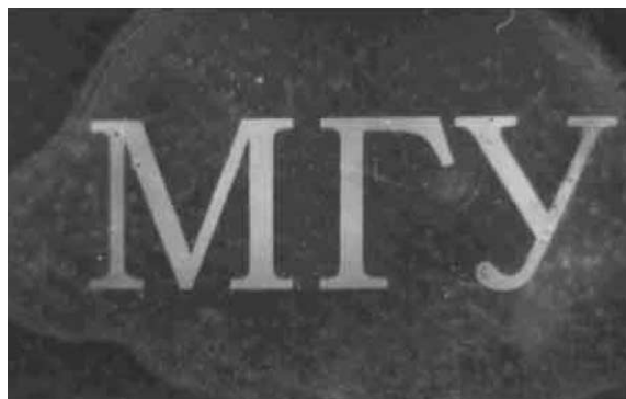
Fig. 41. Microphoto of the film prepared from the copolymer 50 with 15 mol% of chiral-photochromic units exposed to UV-irradiation (365 nm, 15 min). In the figure the red characters which mean Russian abbreviation of Moscow State University corresponding to the irradiated zones are clearly seen on the blue background of the initial sample [46].
