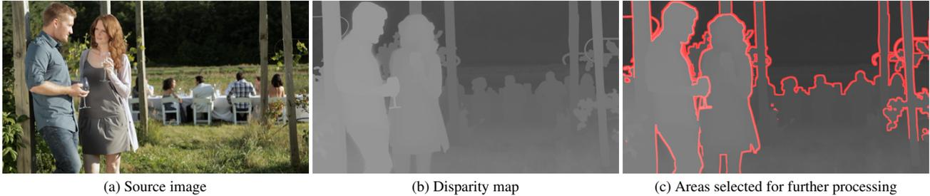
**Fig. 2.** Example of input data for the proposed method: (a) source image and (b) disparity map. The first step involves estimating the mask (c) of pixels along the disparity-map edges (the example shows an estimated mask, in red, over the original disparity map).
