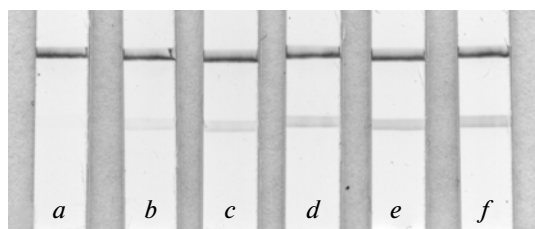
Fig. 3. Results of the determination of the standard h-FABP solutions, ng/mL: a, 0; b, 5; c, 10; d, 20; e, 50; and f, 100.
