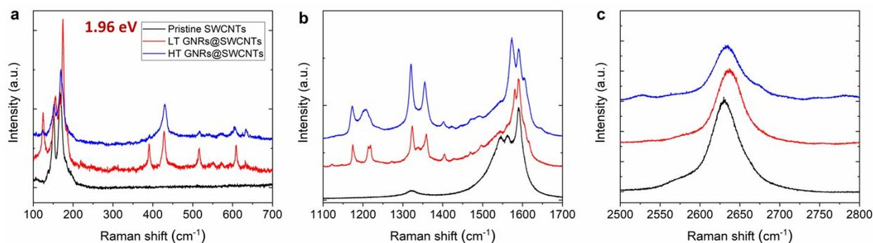
S2 Raman spectra of the pristine SWCNTs (black), low temperature grown GNRs inside SWCNTs (red) and high temperature grown GNR inside SWCNT (blue). Excitation wavelength 1.96 eV.
