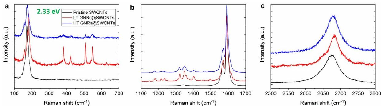
S1 Raman spectra of the pristine SWCNTs (black), low temperature grown GNRs inside SWCNTs (red) and high temperature grown GNR inside SWCNT (blue). Excitation wavelength 2.33 eV.
