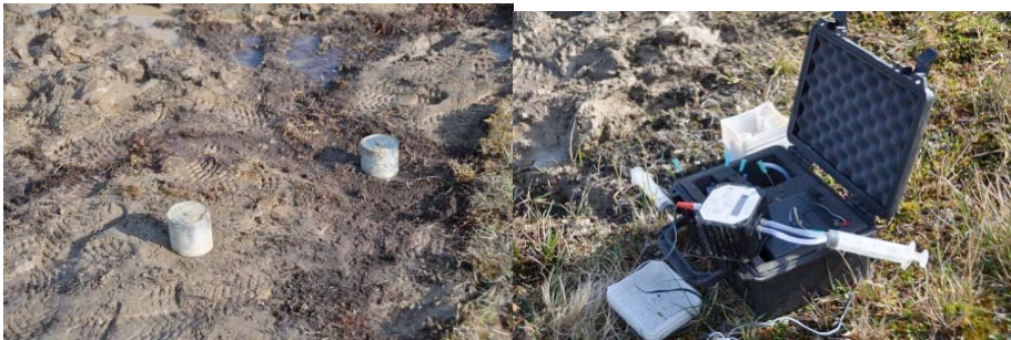
Sampling CO 2 emission from cracks and center of polygons.
