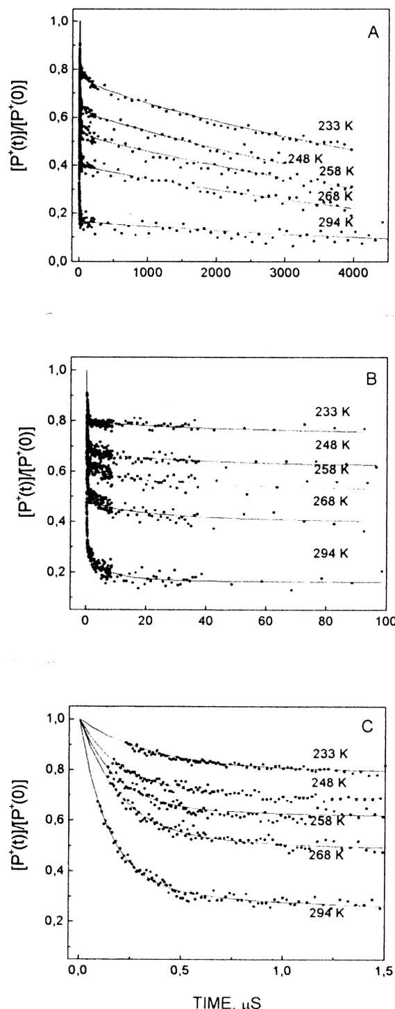
Fig. 1. Kinetics of normalised flash-induced absorption changes at 1283 nm of the cation-radical  $P^+$  in RC from *Rps. sulfoviridis* for the first state of cytochrome reduction ( $E_h = +360$  mV) at different temperatures on different time scales. Solid circles: experimental measurements; line graphs: fitting according to the model described in the paper. (A) Full time scale; (B) 100  $\mu\text{s}$  time scale; (C) 1.5  $\mu\text{s}$  time scale.
