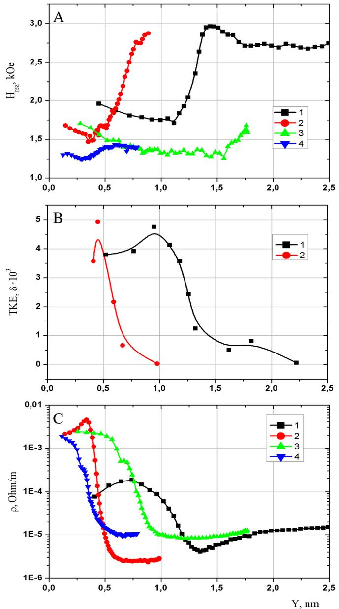
Fig. 1. Dependences of  $H_{rez}$  (A), TKE (B) and resistance  $\rho$  (C) on the thickness of Si layers.
