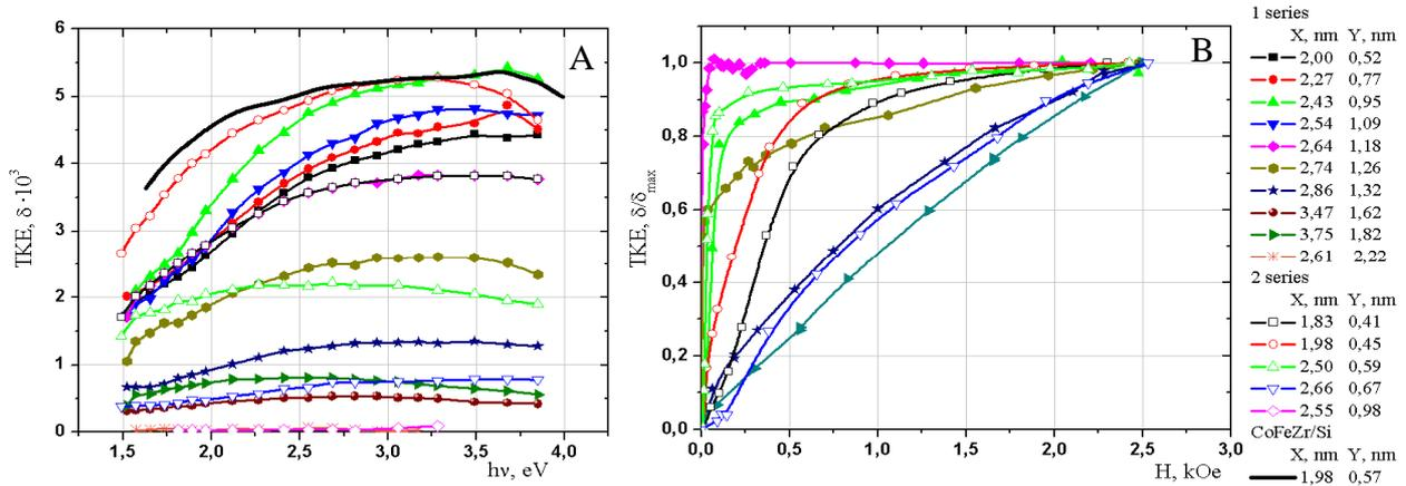
Fig. 2. Spectral (A) and magnetic field dependences of TKE (B) for 1<sup>st</sup> and 2<sup>nd</sup> series ML
