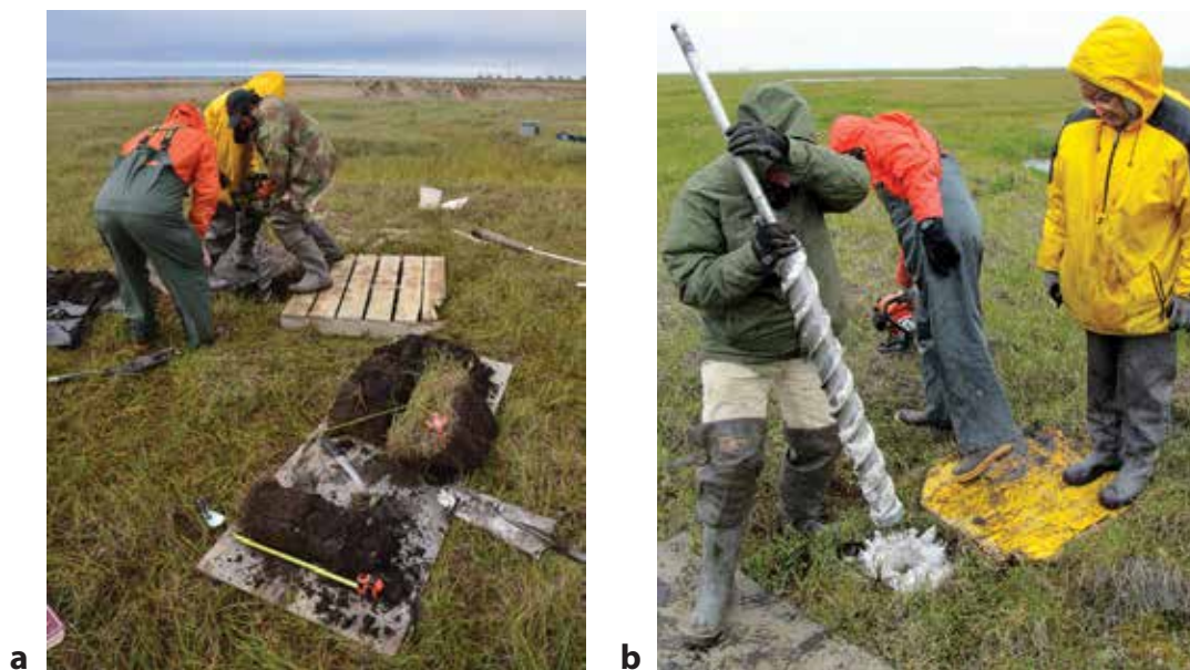
Figure 5.10. (a) Coring a polygon center on the southwest side of the road. Before drilling the vegetation was described and a soil plug was extracted as in the foreground. Sheets of plywood and wooden pallets were used to protect the tundra. (b) Extracting the drill and core from a borehole in a polygon trough ice wedge.
