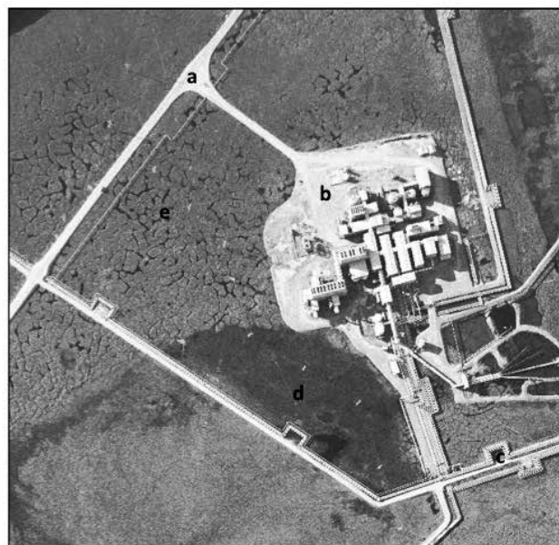
Figure 4.3. Examples of direct infrastructure-related effects: (a) road, (b) pad, (c) pipelines; and indirect effects: (d) flooding due to impeded drainage, (e) permafrost degradation due to altered drainage patterns—in a 1-km 2 area of the Prudhoe Bay Oilfield, Alaska, as seen on 2010 aerial photography. Other indirect effects are visible at full resolution, including: powerlines (one crosses from upper left to lower right, passing near (d)), trails in lower left corner, and gravel and dust adjacent to the road in upper left. This site is located in Map B (Fig. 4.2), near letter (n) in Figure 4.8.
