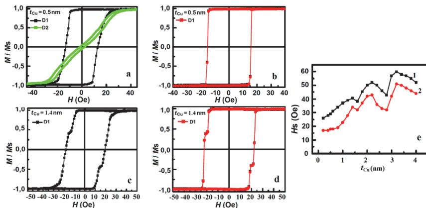
Figure 2. Hysteresis loops of Co/Cu/Co samples measured employing magneto-optical (a, c) and vibration sample (b, d) magnetometers; (e) dependences of  $H_S(t_{Cu})$  obtained by using the data of magneto-optical (curve 1) and vibration sample magnetometers (curve 2).
