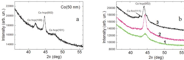
Figure 1. X-ray spectra observed for the reference 50 nm Co film (a), and the samples contained Ta, Co and Cu (b): curve 1 – Ta/Co(5 nm)/Ta, curve 2 – Ta/Co(5 nm)/Cu(1 nm)/Co(5 nm), curve 3 – Ta/Co(5 nm)/Cu(4 nm)/Co(5 nm).
