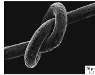
Figure 1. Image of the thick \text{Co}_{69}\text{Fe}_4\text{Cr}_4\text{Si}_{12}\text{B}_{11} microwires, illustrating its ability to tighten into a knot without fracture.
