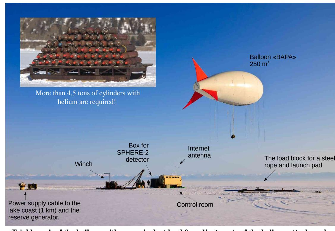
Trial launch of the balloon with an equivalent load for adjustments of the balloon attack angle.
