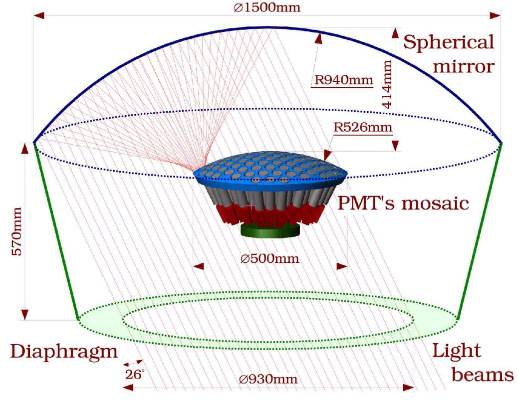
**Optical scheme of the SPHERE-2 detector**
