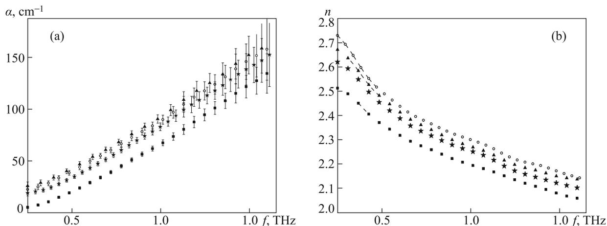
Spectra of (a) absorption coefficients and (b) refractive indices of (▲) water, (○) blood plasma of control rats, (★) blood plasma of rats with diabetes, and (■) glucose solution.
