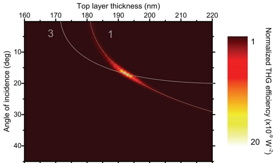
Fig.1. Efficiency of THG in PC/Me sample for *pp* combination of fundamental and TH radiation polarizations, versus the angle of incidence and thickness of the topmost layer of a PC. Gray curves are guides for the eye and represent dispersion curves of the fundamental (1, dashed) and third-order (3, solid) Tamm plasmons.
