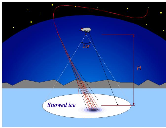
Scheme of the experiment with tied balloon on Baikal lake. The surveyed area ~0.75H<sup>2</sup>
