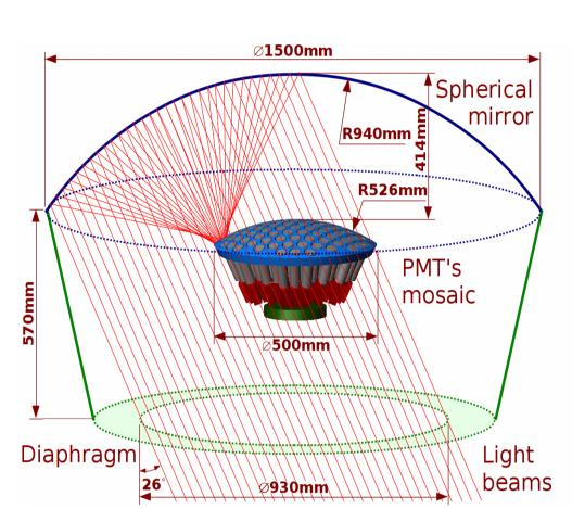
Optical scheme of the SPHERE-2 detector.
