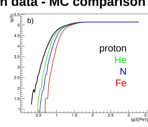
instrumental Simulated acceptance for 2013 data conditions for different nuclear
