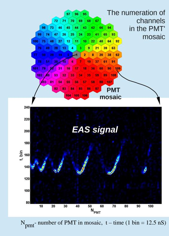
Amplitude of the curve correlates with zenith angle, phase shift reflects the azimuthal angle.
