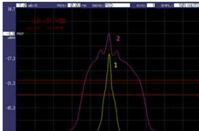
Fig. 3. Spectrum Optical signal spectrum at the output of the optical fiber without an amplifier (1) and with an amplifier (2)
