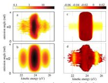
Experimental (a,c) vs theoretical (b,d) cross section (a,b) and circular dichroism (c,d) in He 1s 2color photoionization. The dichroism is a direct measurement of the degree of circular polarization.
