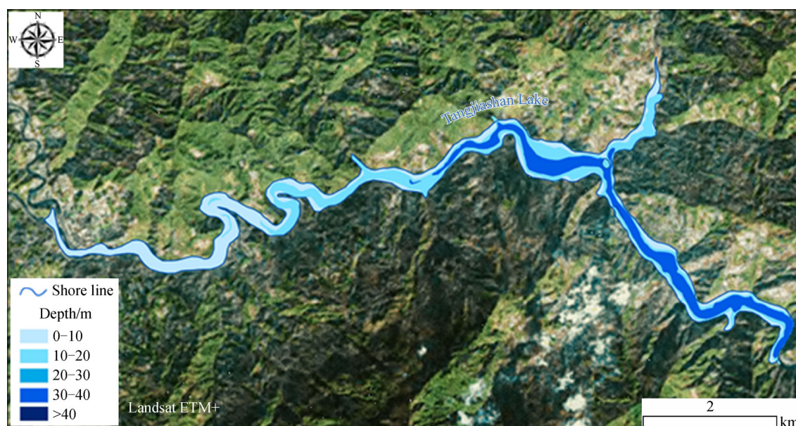
Fig. 5 Tangjiashan Lake depth according to bathymetric surveys (background image: Landsat ETM+).
