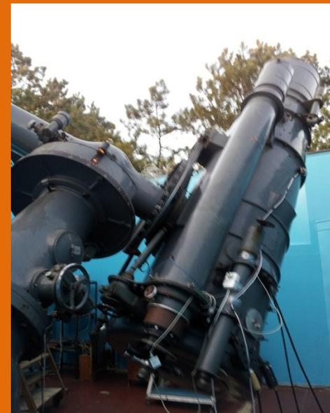
50 cm meniscus Maksutov telescope AZT-5. Field  $3.7 \times 3.7^\circ$ , scale  $103''/\text{mm}$ , exposures of 60 min, plate limit  $\sim 20$  mag
