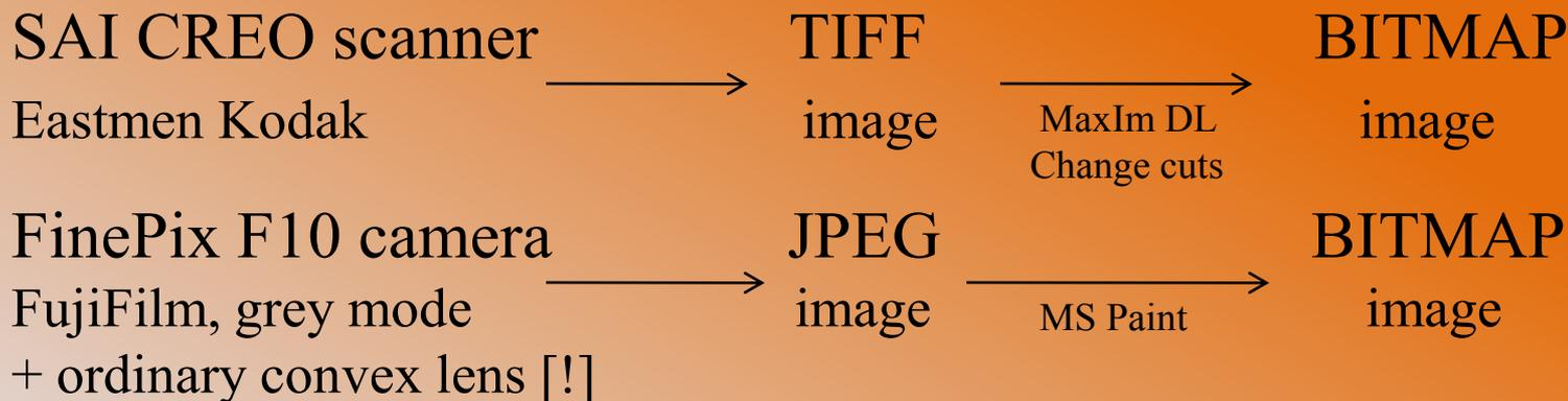
The second method can't be used for wide fields due to lens distortion but is good for a single star with outskirts. It may be widely used by students and amateurs even without support stands.
