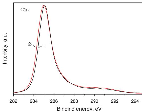
**Fig. 6.** C1s core level of pristine SWNT (**1**) and [Mo]-SWNT (**2**).
