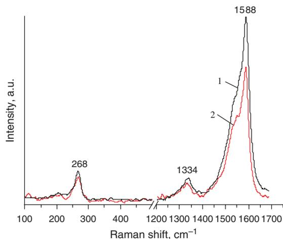
**Fig. 4.** Raman spectra ( $\lambda_{\text{ex}} = 514.5$  nm) of pristine SWNT (**1**) and [Mo]-SWNT (**2**).
