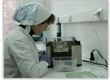
3. Assembling of a multimembrane composite and cutting it into individual test strips
