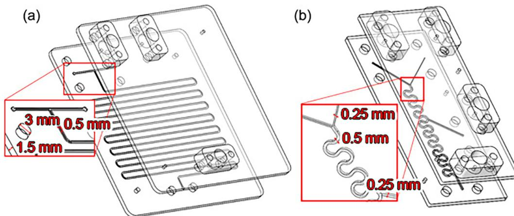
**Scheme 33.** First (a) and second (b) stage reactors. (Reactor tube diameters vary from 0.25 to 0.5 mm). Reproduced with permission [96], Copyright 2017, John Wiley and Sons GmbH.
