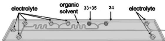
Fig. 7. Reagent injection scheme for the microchip [47,48].
