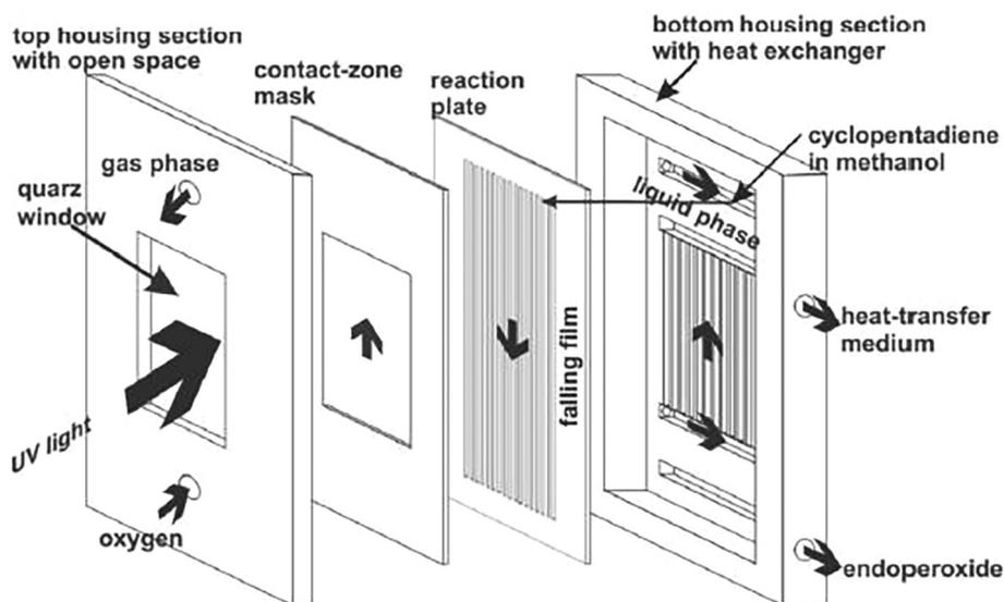
Fig. 5. Photooxidation microchip construction [55].
