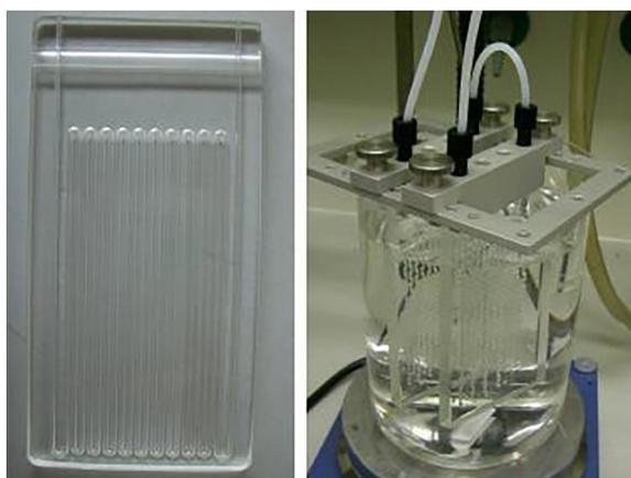
Fig. 3. Chemtrix microreactor cell. Reproduced with permission [47,48]. Copyright 2012, Beilstein-Institut.
