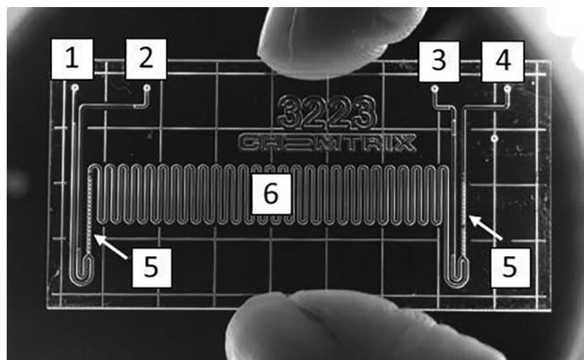
Fig. 2. Chemtrix type 3223 microfluidic reactor.
