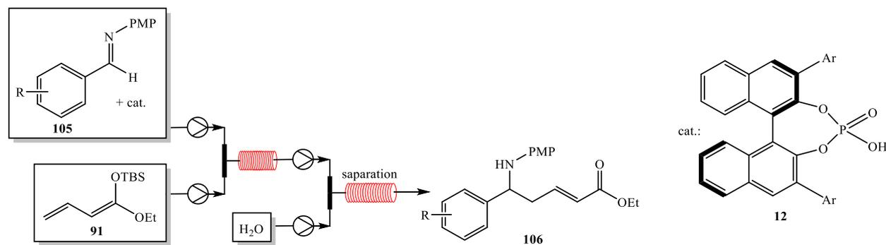
Scheme 25. Integrated Mannich reaction apparatus [47].
