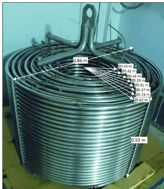
Fig. 4. Pilot plant for the intermediate production in the synthesis of «LY500307». 73 Liter continuous flow reactor [51]. Copyright 2012, American Chemical Society.
