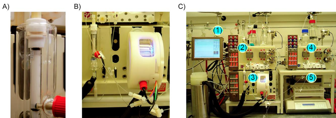
Fig. 8. General reactor setup. (A) A glass Omnifit column is packed with 1 g of proline. (B) The column is then placed in-line with a 10 mL PFA coiltube reactor (3). (C) The components are connected to HPLC pumps (2, 4) for solvent and reagent inputs. The reactor is controlled by a computer (1) in order to program the timing of the reagent and solvent inputs and fraction collection (5). Reproduced with permission. [87] Copyright 2011, Beilstein-Institut. Vapourtec R series reactor system [88].
