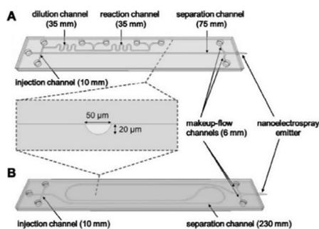
**Fig. 6.** Flow-through reactor for enantioselective Mannich reaction [47].
