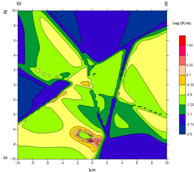
**Fig. 2. Horizontal conductivity cross-section at the depth 5.25 km b.s.l.**
