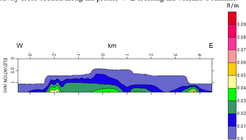
**Fig.1. The vertical conductivity cross-section along WE profile revealed by ANN inversion of MT data.**
