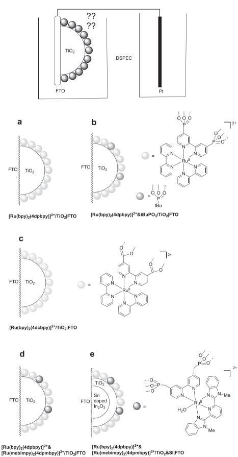
Fig. 1. Various photoanodes for organic synthesis in DSPECs (only one TiO<sub>2</sub> nanoparticle of mesoporous nanostructured films is shown).
