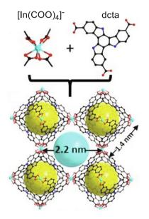
Fig. 2. Structure of PCN-99. Reprinted with permission from Ref. [54]. Copyright 2016 Royal Society of Chemistry.
