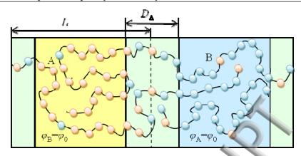
FIG. 1. Schematic of a segregated melt of the random multiblock copolymer with  $N_{\rm sh}=1$  and  $N_{\rm long}=6$ .
