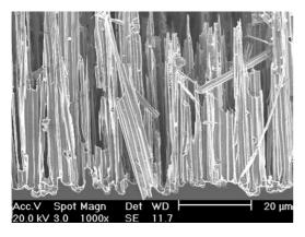
Figure 1. Silicon wires obtained by one-step chemical etching.
