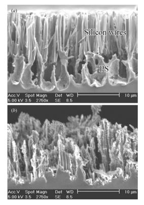
**Figure 2.** Different structures after electrochemical anodization (*a*) porous silicon covered with silicon wires by using thinner silicon wires; (*b*) PS-covered wires by using thicker (over 1  $\mu$ m in diameter) Si wires.
