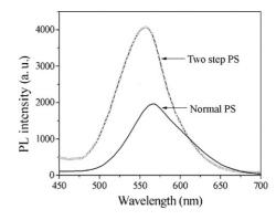
Figure 3. Photoluminescence spectra of normal PS and two-step PS.
