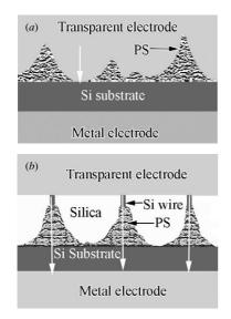
**Figure 4.** Schematic drawing of electric contacts in devices fabricated on top of (*a*) normal PS and (*b*) PS connected with silicon wires.
