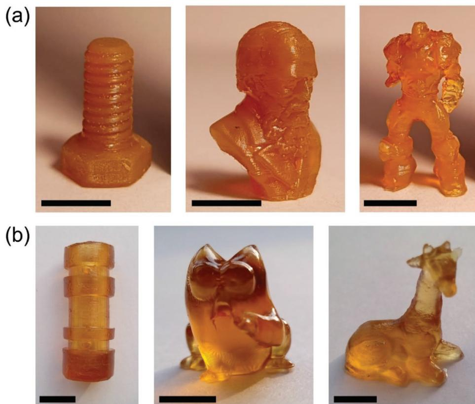
**Figure 8.** Examples of 3D structures fabricated from a) OPBI-PSC and b) MPA-PSC by DLP 3D printing. Scale bar is 5 mm.
