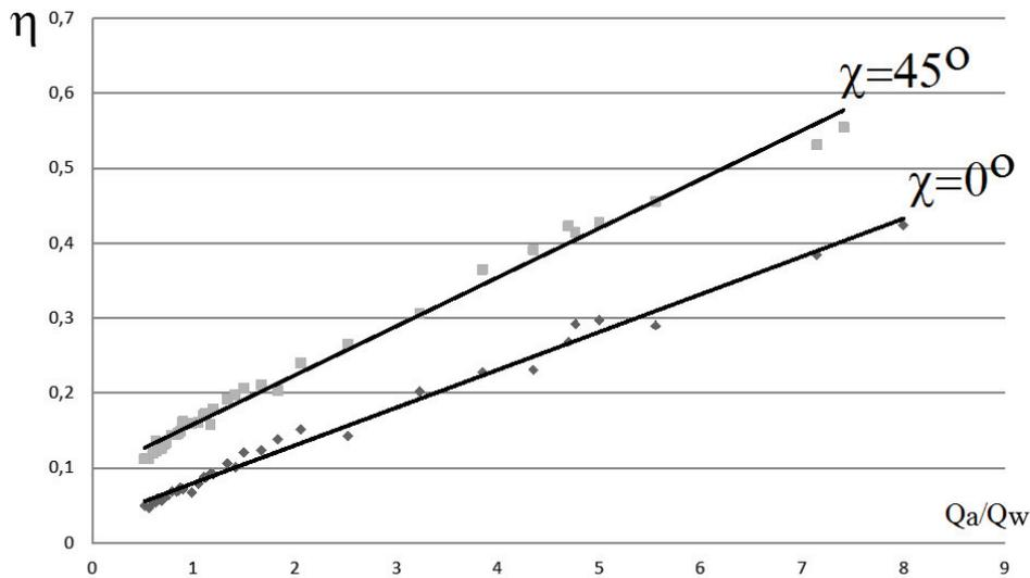
Fig. 3. Change of the tower thermal efficiency ratio against relation between air-dynamic and hydraulic loads  $Q_a/Q_w$  in case of open cooling tower and the tower with flow vortex along whole perimeter by air-regulating devices.
