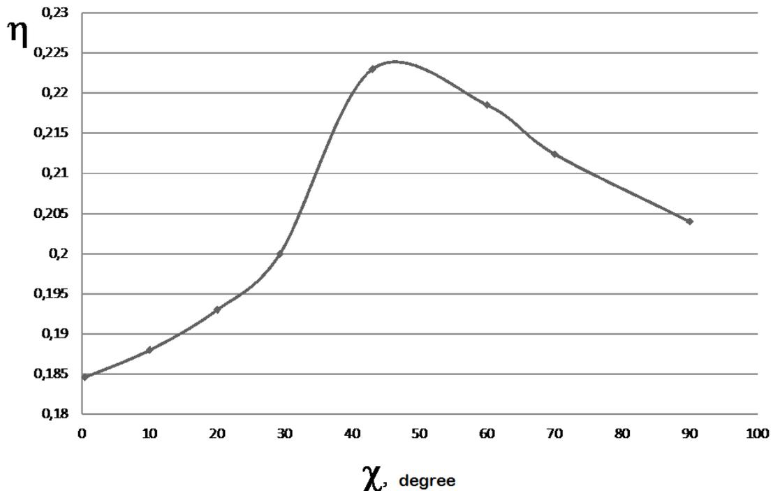
Fig. 2. Plot of the efficiency ratio dependence at given air flow input angle  $\chi$  from 00 to 900 and relative flow rate  $Q_a/Q_w=1.1$ .
