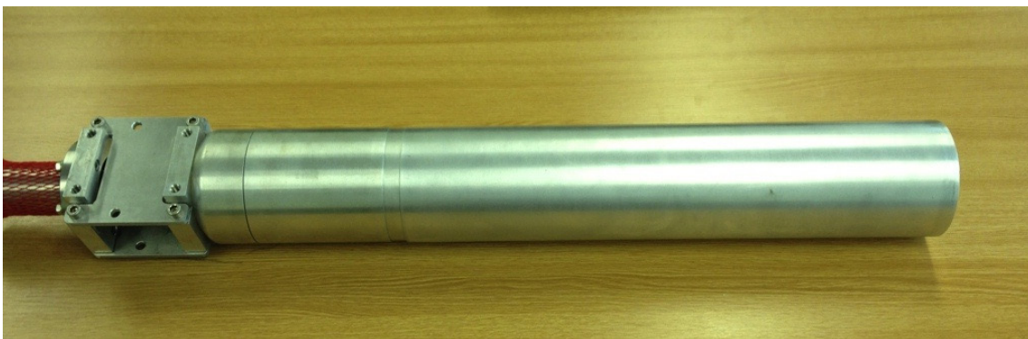
FIG. A-7. The N-Visage scanner (cylindrical component) mounted on a deployment tool. OD is 110 mm.
