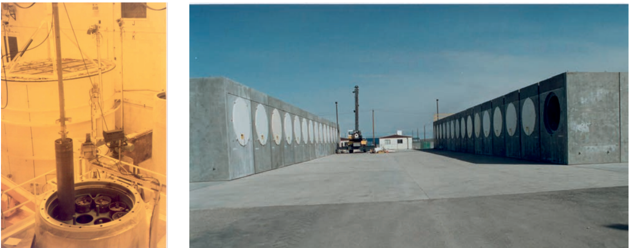
FIG. 19. On the left, TMI-2 fuel debris drying; on the right, placement in dry storage.
