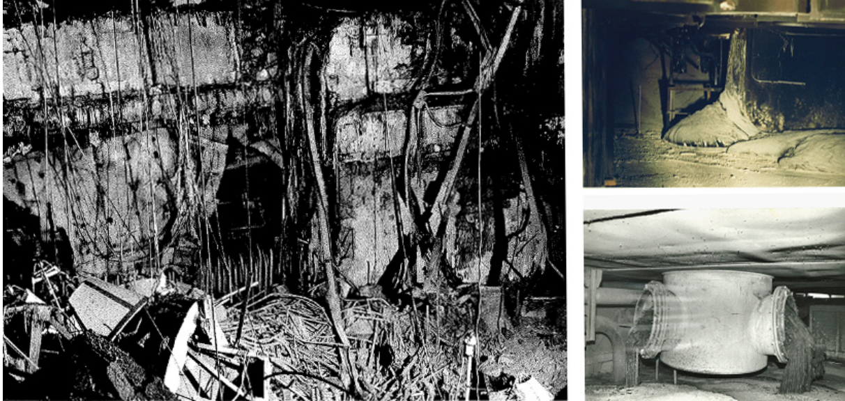
FIG. 12. Chernobyl core cavity and corium.
