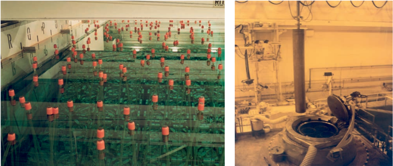
FIG. 18. On the left, the storage pool at TMI-2; on the right, the loading of a canister into the heated vacuum drying oven.
