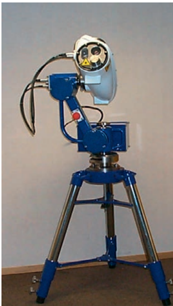
FIG. A-6. The RadScan 800 device (left) and images of ^{137}\text{Cs} contamination in a nuclear facility (right).
