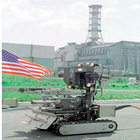
FIG. A-5. The Pioneer remote reconnaissance system.
