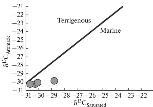
Fig. 6. The distribution of the  $\delta^{13}\text{C}$  ratio of the aromatic and saturated HC fractions.
