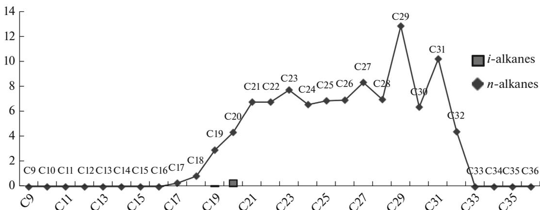
Fig. 5. The distribution of *n*- and *i*-alkanes according to the results of gas–liquid chromatography of sample H12-10b.
