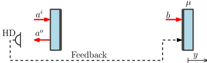
Fig. 1. Scheme of Fabry-Perot cavity with movable mirror (rightmost one).
