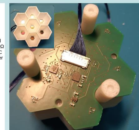
Diagram of SiPM segment. The negative SiPM supply voltage is common to all 7 channels, and the positive voltage can be set separately for each channel. An LMT70 temperature sensor have an accuracy of ±0.23 °C is installed next to each SiPM. A cascade of two amplifiers generates an output pulse for FADC with FWHM of 20-25 ns and amplitude of up to 3.5 mV / photoelectron.
