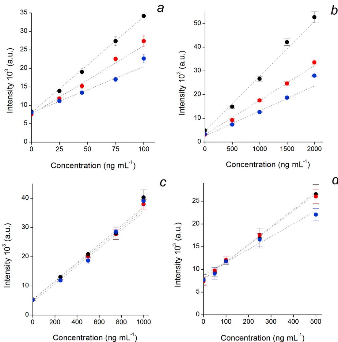
**Fig. 3.** Calibration curves for a) Myo, b) Cys-C c) CRP and d) D-Dm spiked samples at different incubation time: 10 min (black), 5 min (red), 3 min (blue) for myoglobin, cystatin-C, CRP and 15 min (black), 10 min (red), 5 min (blue) for D-dimer. (For interpretation of the references to colour in this figure legend, the reader is referred to the Web version of this article.)
