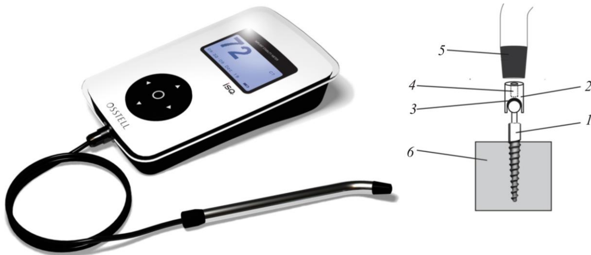
Fig. 3. Measurement design for quotients of longitudinal stability of mini dental implants using Osstell ISQ device: 1 is mini implant; 2 is measuring cap; 3 is temporary cement layer; 4 is magnetic element of the measuring cap; 5 is probe of the Osstell ISQ device; 6 is osseous tissue)
