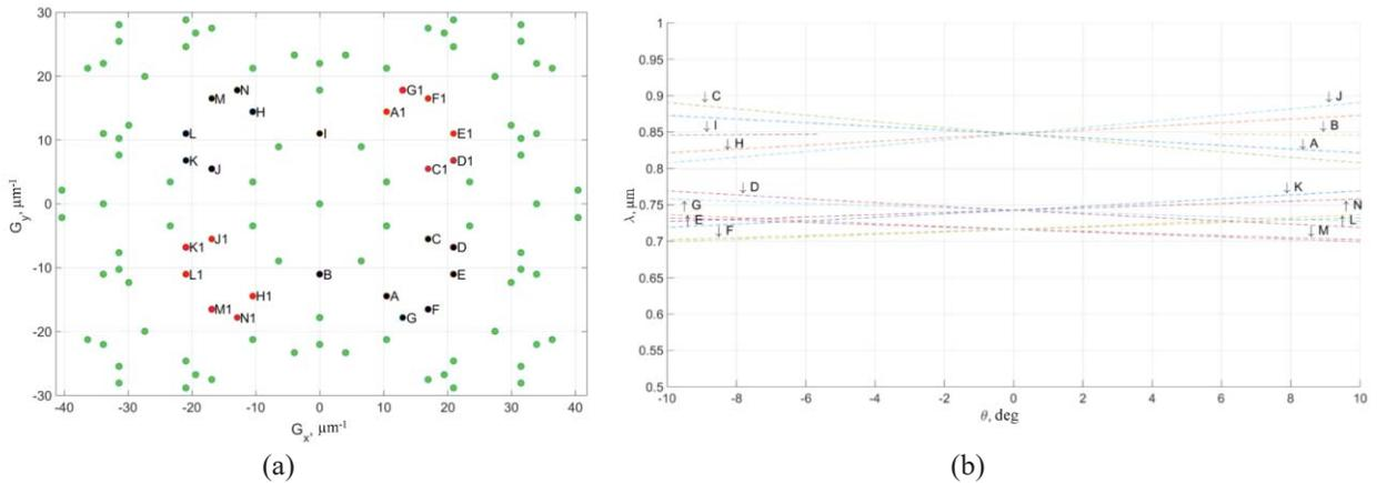
**FIGURE 1.** The reciprocal lattice vectors (a) and dispersion diagram (b) of 2D quasicrystal
