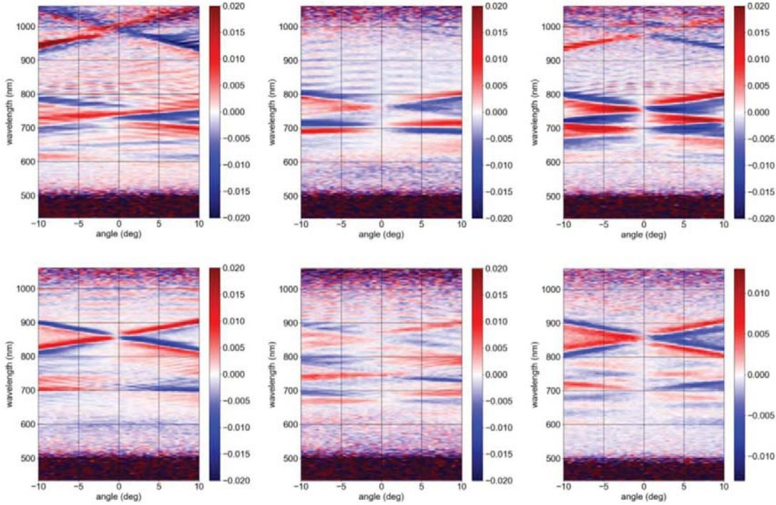
**FIGURE 2.** The TM-polarized light's TMOKE spectra (upper row: two-dimensional plasmon crystals with angles  $\pi/2$ ,  $\pi/3$ ,  $\pi/4$ ; lower row: crystals with angles  $\pi/5$ ,  $2\pi/5$  and a two-dimensional quasicrystal)
