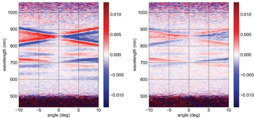
**FIGURE 3.** TMOKE spectrum in a 2D magnetoplasmonic quasicrystal with TM and TE polarization of incident light
