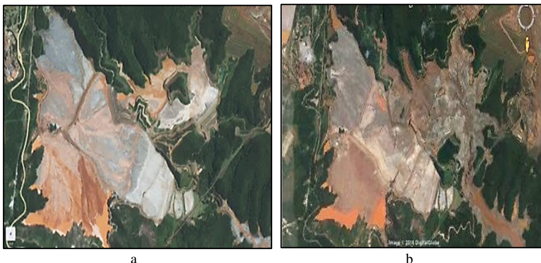
Fig. 1. Fundão Dam and Reservoir; (a) during construction and before rupture, and (b) after rupture and upon emptying of the reservoir
