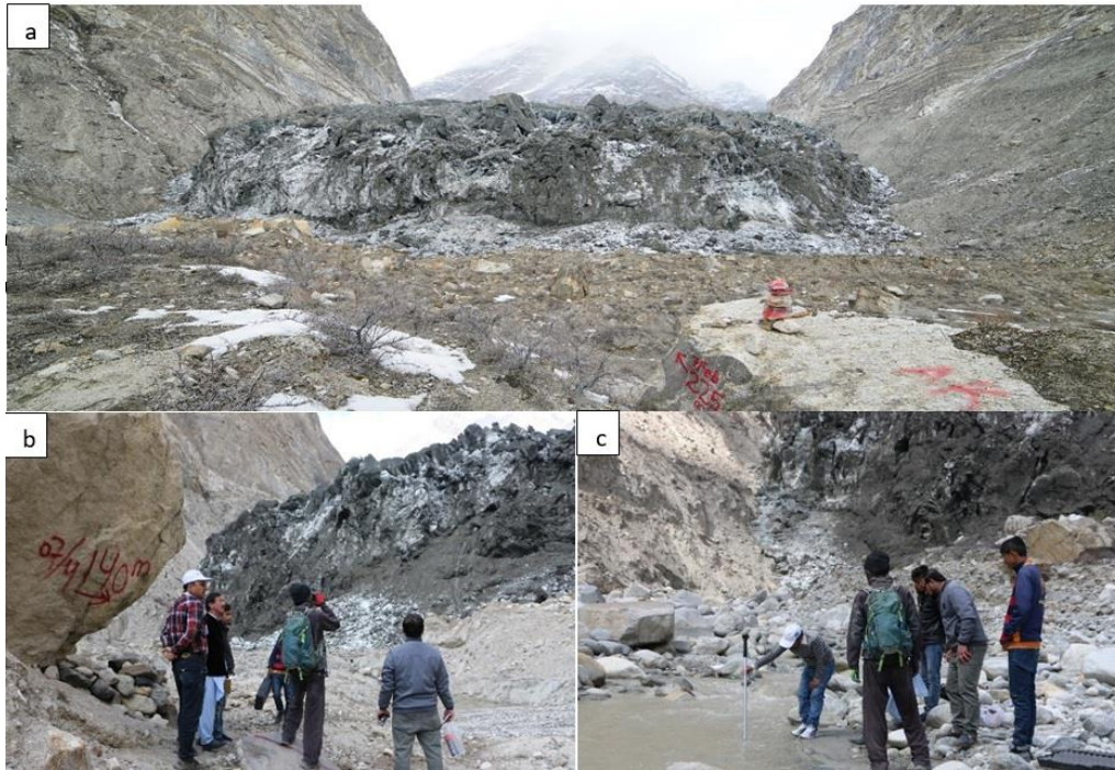
Fig. 3. a) Frontal view of snout and marked boulders for monitoring rate of glacier surge. b) CERT team taking measurements from the benchmarks during the training. c) AKAH geologist measuring velocity of water near snout by velocity meter while CERT team observing. Photo credit AKAH Pakistan
