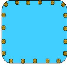
Fig. 2. Monolith conductor layout, size 113 mm  $\times$  113 mm, for an 80-kA nominal current in a 50-GJ solenoid, 20 m long, and providing 6 T in a 12-m bore.
