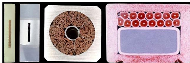
Fig. 1. Characteristic conductor layouts used in the present large-scale magnet like ATLAS and CMS detector magnets; ITER PF coils and LHD.
