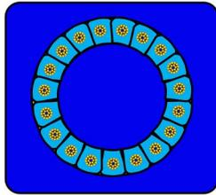
Fig. 3. CICC conductor layout 80-kA nominal current in a 50-GJ solenoid. Subcables included in an SS304 structure, outer size 90 mm  $\times$  91 mm.
