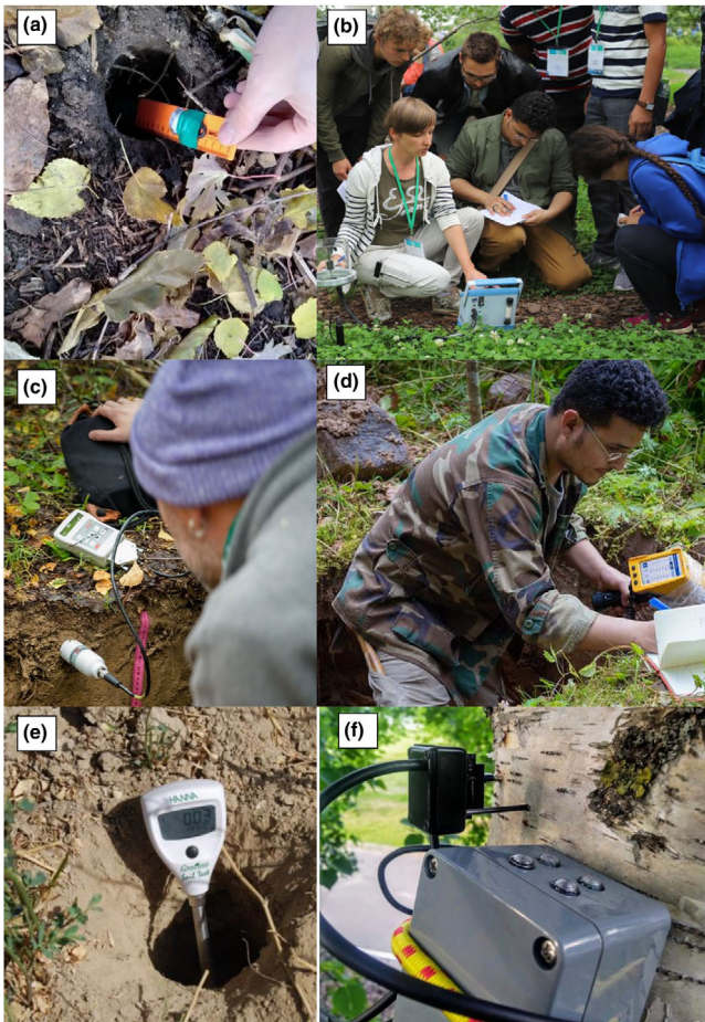
FIGURE 3 Mastering skills in advanced techniques of soil and plant monitoring by using (a) portable temperature sensor iButtons, (b) infrared gas analyzer (IRGA), (c) soil moisture probe SM-300, (d) portable X-ray fluorescence (XRF) analyzer, (e) electrical conductivity (EC) meter and (f) Tree Talker
