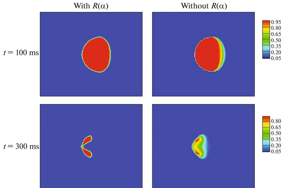
Fig. 4. Distribution of the volume fraction of gas in the problem of a shock wave interaction with a gas bubble.
