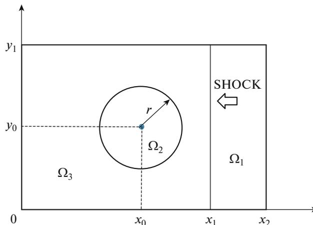
**Fig. 3.** Diagram of the problem of a shock wave interaction with a gas bubble.
