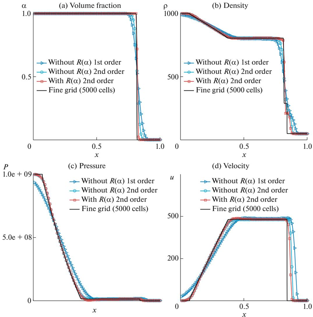
Fig. 2. Numerical solutions of the shock tube problem.
