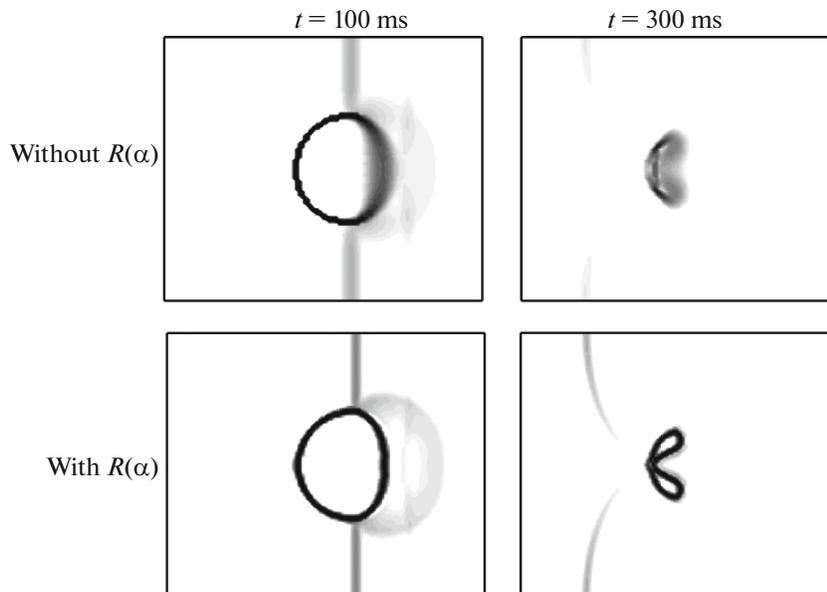
Fig. 5. The field of the gradient density (numerical schlieren) in the problem of a shock wave interaction with a gas bubble.
