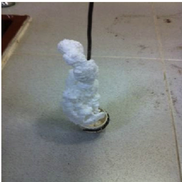
Fig. 1. \text{SrAl}_2\text{O}_4:\text{Eu}^{2+} (1%) ash synthesized by combustion method.
