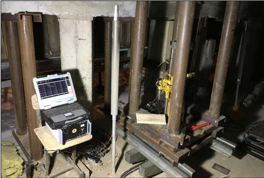
**Figure 7:** Mobile CPT Equipment during Testing (TCPT-04)
