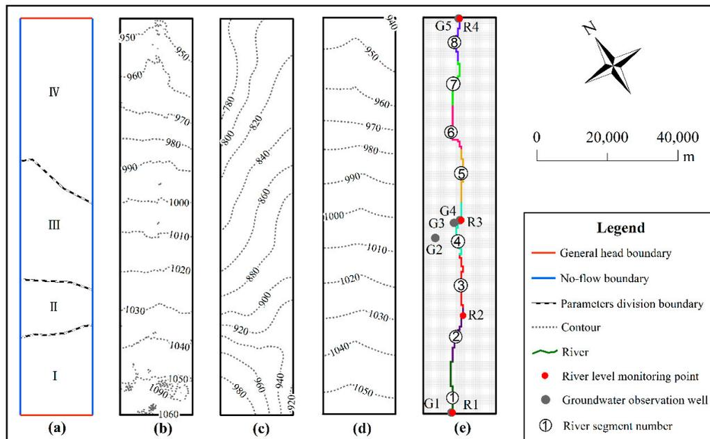
**Figure 2.** Model setup: (a) parameter division; (b) land surface elevation; (c) bottom elevation of the aquifer; (d) initial water levels; and (e) river segment division and monitoring sites.
