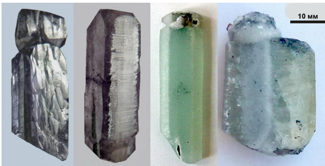
Fig. 1. External morphology of topaz single crystals grown in supercritical water-fluoride solutions.
