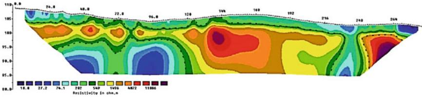
Fig. 5 Model of electrical resistivity
