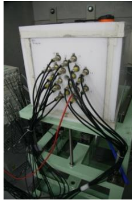
Fig. 18 - Neutron detectors installed at the gamma beam line GACKO.
